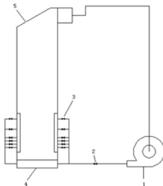
1. Fan 2. Valve 3. Burner 4. Air Chambe 5. Furnace
